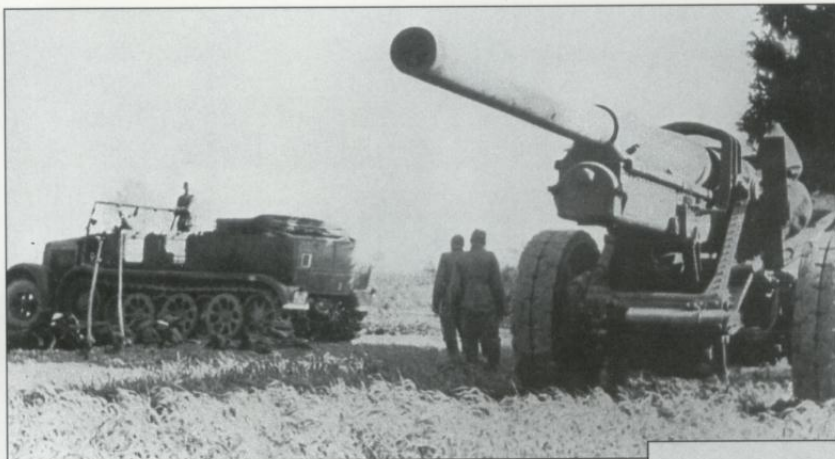
Another type of heavy artillery, a 15cm gun, this time with a much more powerful "team", the 8-ton Sd.Kfz. 7 tractor. This photo clearly illustrates the dimensions of this type of weapon. Note the tactical marking on the vehicle.
