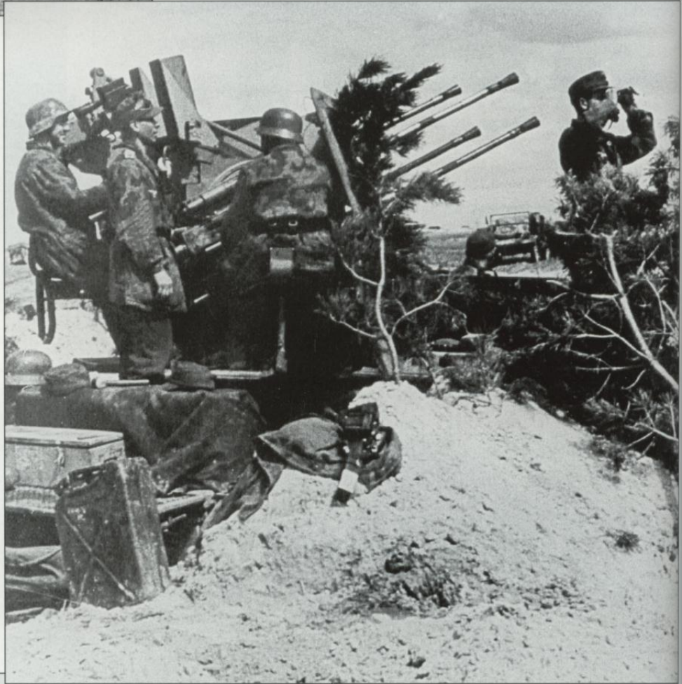
Waiting for enemy air attack. A Luftwaffe gun crew wearing camouflaged uniforms is ready to go into action with its 2cm Flakvierling 38 anti-aircraft gun, which is installed on a Sd.Kfz. 7 vehicle. The gun is equipped with the early version armored shield.
