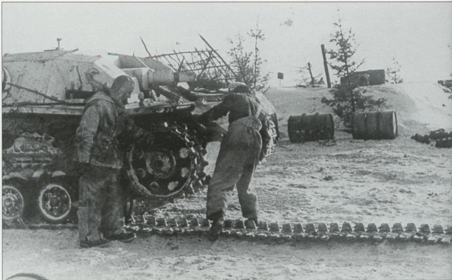
Under cover of an 8.8cm Flak gun (visible in the background in a specially prepared position), StuG crew members repair the damaged tracks of their vehicle. The winter camouflage on the StuG III is worn only on the superstructure and the front part of the hull. The small ring on the StuG's gun barrel is a dark gray color.
