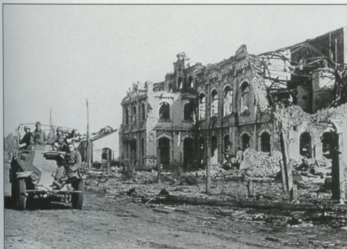
A lone Sd.Kfz. 261 light armored radio car passes by a destroyed industrial building in a town somewhere on the road to Moscow. The first half of the distance to Moscow was covered by the Panzerwaffe troops without excessive difficulty. The Sd.Kfz. 261s were issued to the signal troops of the headquarter units.
