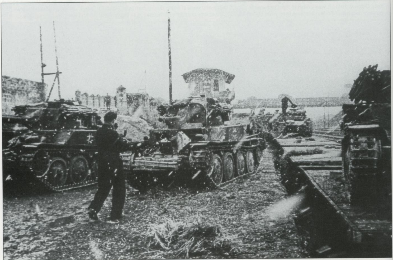
This photo shows the reloading of Pz.Kpfw. 38(t)s that have bundles of wood attached to their turrets and the front of their hulls. Petrol cans and boxes were stored at the rear of the turret. Such heavily equipped turrets were not commonly seen in units armed with these tanks, and such sights were probably limited to October 1941. The first wet snow fell on 5th October. During the next few days combat conditions changed very much.
