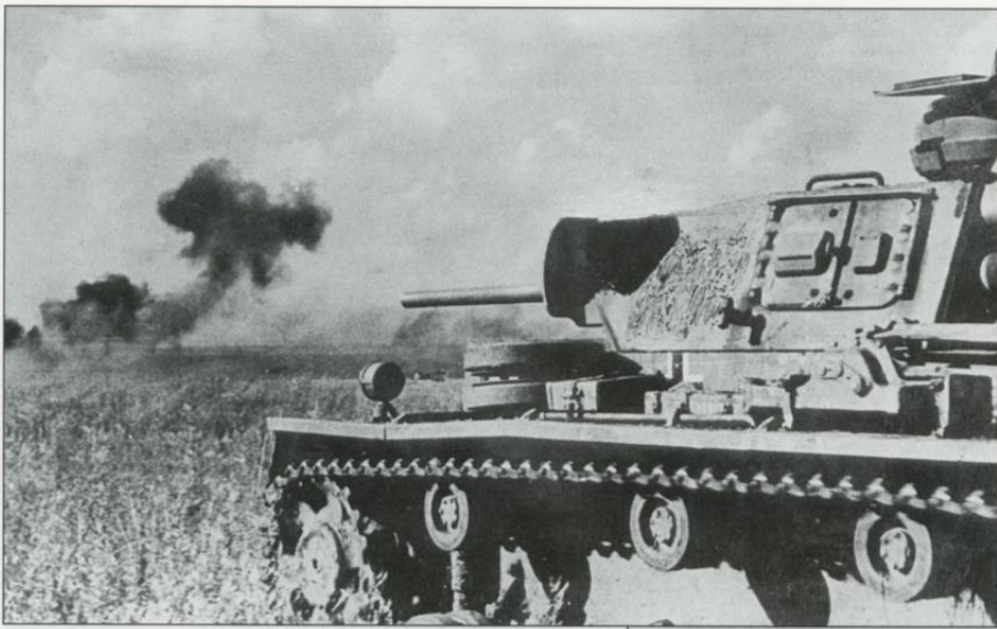
This close-up photo of a Pz.Kpfw. III Ausf. L shows very well the shape of the additional armor on the front of the turret and the length of the new 5cm KwK39 gun. The tactical number of the vehicle was censored. This model of Pz.Kpfw. III was first produced in June 1942.
