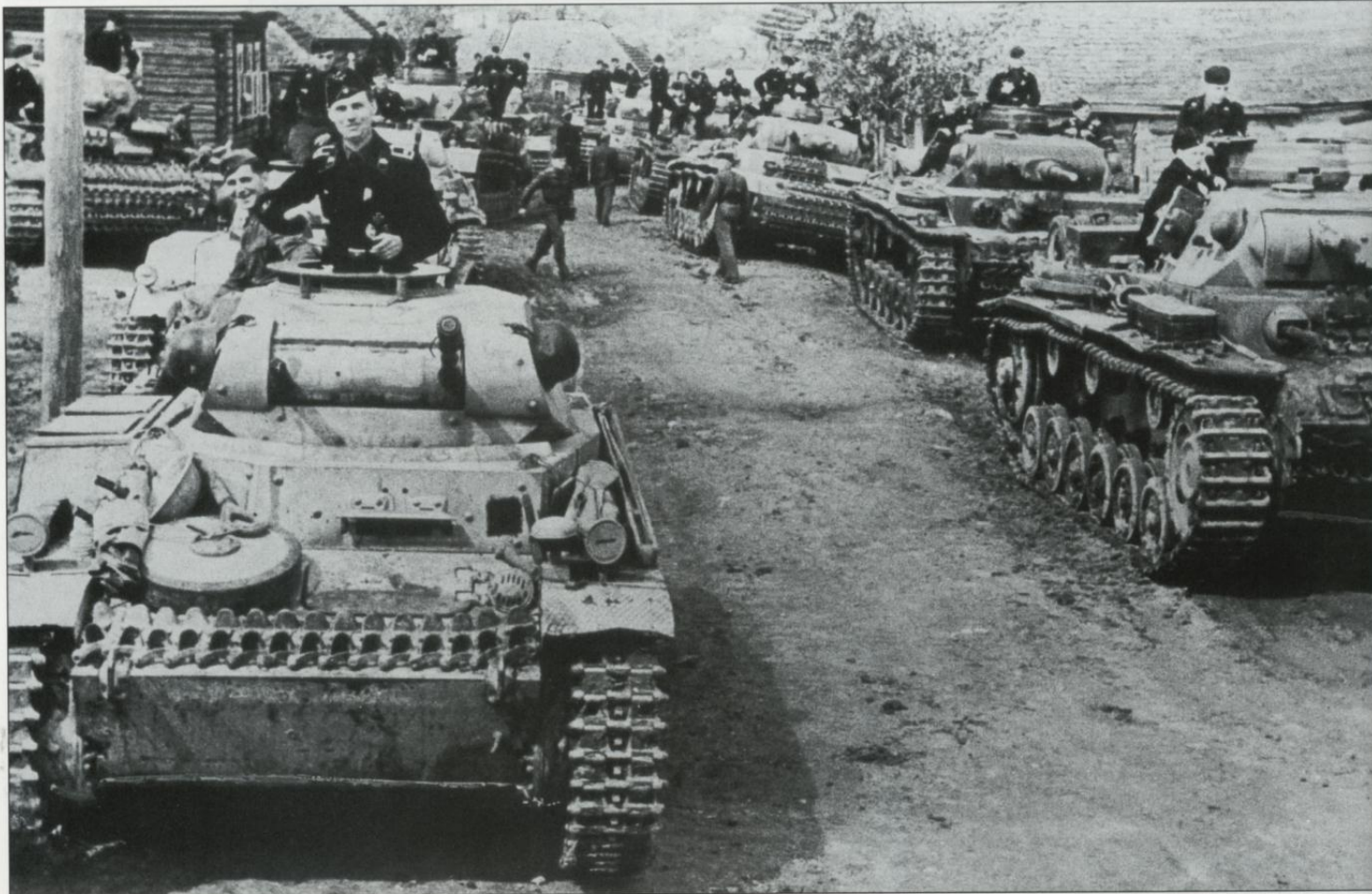
The main support units for the October offensive against Moscow (Operation "Typhoon") were two new divisions from the OKW reserve, the 2. and 5. Panzerdivisions, which were originally prepared for action in Africa, but were sent to Russia in September 1941. Here we see three Pz.Kpfw. IIs, five Pz.Kpfw. IIIs and three Pz.Kpfw. IVs from one of these divisions. Most of them are painted in a very light paint scheme — the dark sand color that was applied to help them blend in with the North African landscape.
