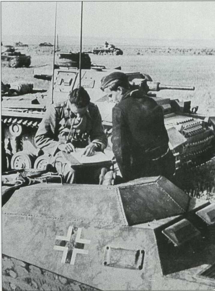
Another strangely modified half-track of 24.Panzerdivision photographed during the advance of divisional armor in the rear areas of the front line. There is no doubt that this is a Sd.Kfz. 250/3 communications vehicle modified by workshops of the division. It is camouflaged with a dark yellow pattern, too. Note that the national cross is somewhat overpainted by the camouflage coat.
