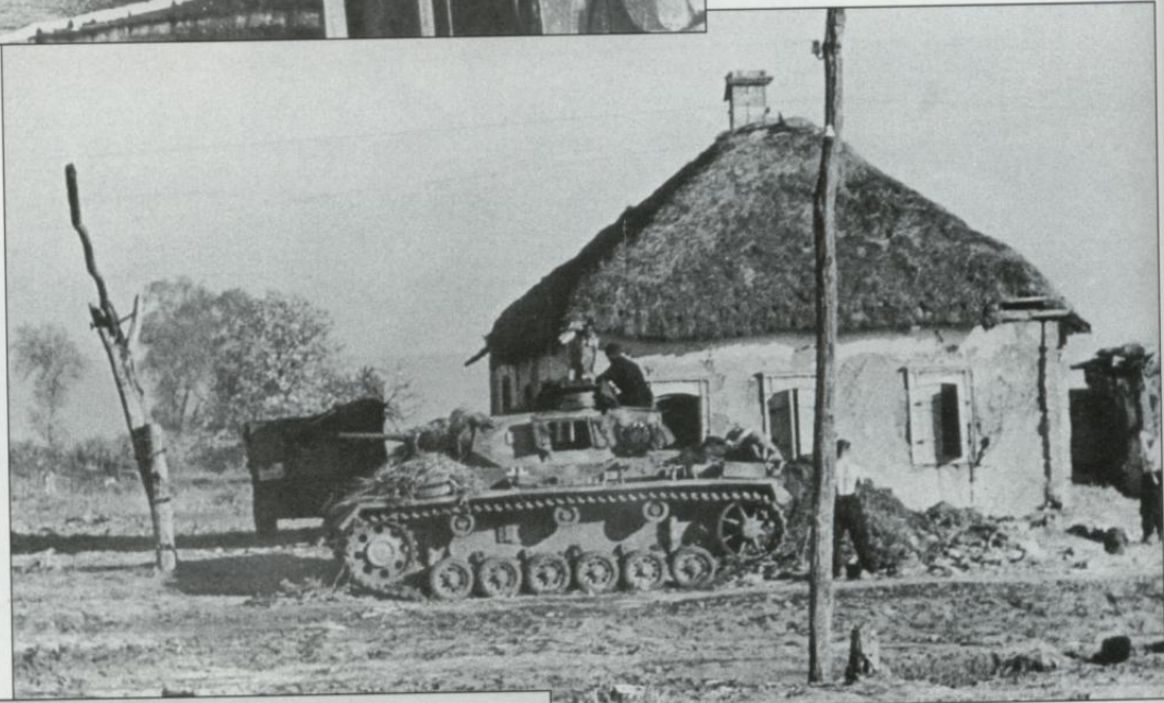
A Pz.Kpfw. III at rest near a hut in Russia. The early Pz.Kpfw. IIIs, with their 3.7cm gun, proved to be inadequate for combat in the early 1940s, even if they were easy to operate and offered good mobility. This type of tank is an excellent example of a "half-way" weapon — much better than light tanks, but not enough good as a medium-size tank.
