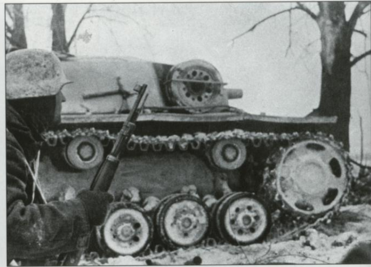
A soldier and a StuG III— two inseparable elements during almost every action on the Eastern Front throughout the war. Note the paint job on the assault gun; white paint has been applied to all the places that were easily accessible between the wheels and the construction and to the hull and superstructure sides.
