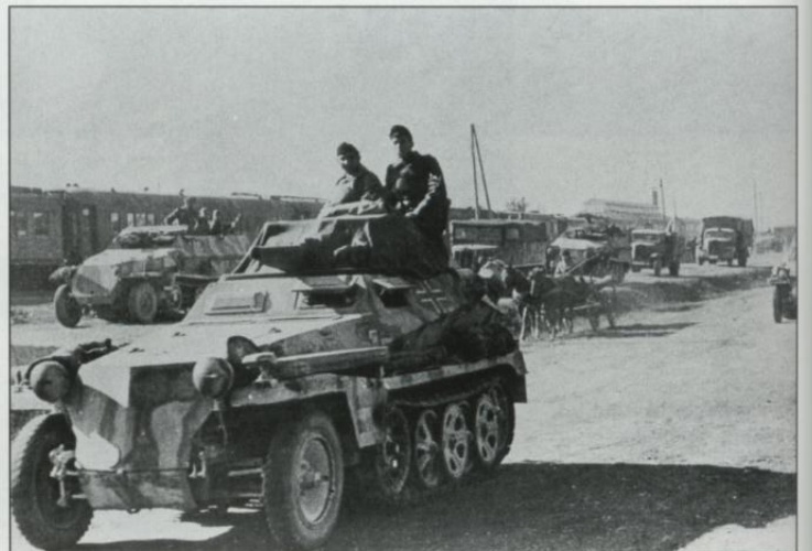
An armored infantry battalion equipped with Sd.Kfz. 250s and Sd.Kfz. 251s (including the artillery model, Sd.Kfz. 251/9, armed with a 7.5cm KwK37 gun) is organized into a column at a train station. All the vehicles are painted with a special pattern of camouflage — green spots outlined with brown on a dark yellow base color. In the background are other such vehicles, as well as soft-skinned supply vehicles.
