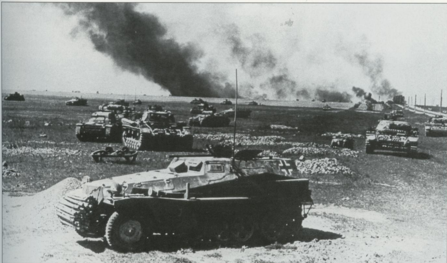
Probably one of the best known photos showing an attack of Panzerwaffe units across open fields. Operation "Barbarossa" opened on 22nd June 1941 with a total of 3,332 German tanks involved. In the foreground is a Sd.Kfz. 253 armored command vehicle, which originally was built for StuG.Abt. (assault gun unit) staffs. Here we see this vehicle as a leading command post of a tank unit composed of Pz.Kpfw. IIs and IIIs and supported by infantry hidden in their Sd.Kfz. 251s.
