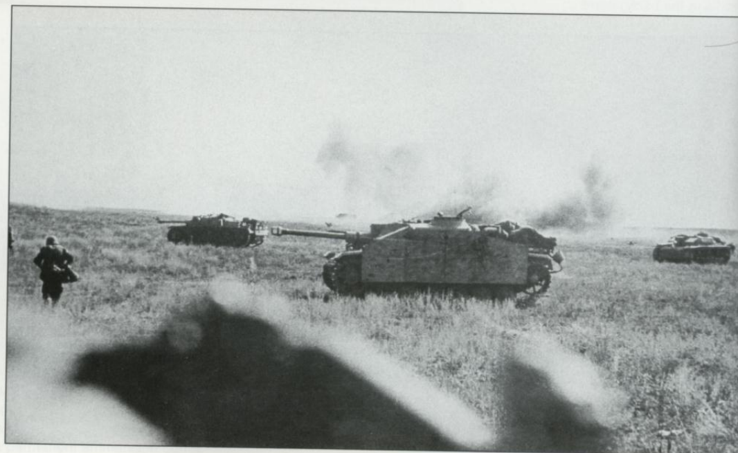
Panzerjäger move into their firing position. This battery is equipped with Marder IIIs armed with Soviet 76.2mm guns and built on the Pz.Kpfw. 38(t) chassis. Note that a censor has blotted out the muzzle breaks. Also of special interest is the vehicle at left. Though it looks like a Marder II, it is probably a munitions vehicle built on Pz.Kpfw. II chassis.
