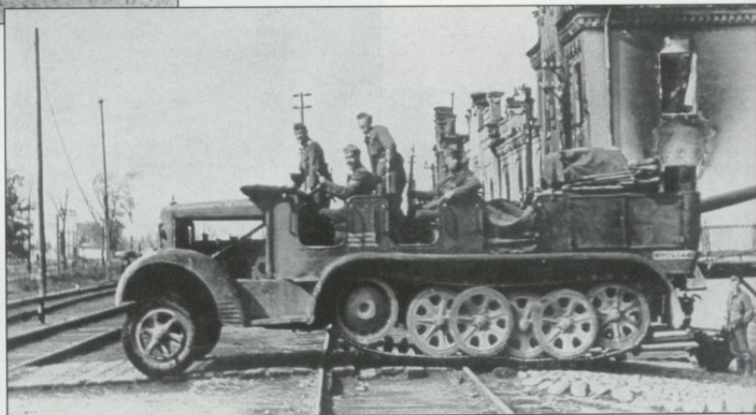
The Germans used five main types of half-tracked tractors for their artillery units. Among them was the 8-ton Sd.Kfz. 7, visible in this photo during a trip to town to obtain supplies. This is the KMm9 version. Note how low the engine is installed. Also of interest is the license plate fixed to the rear of the side of the vehicle.
