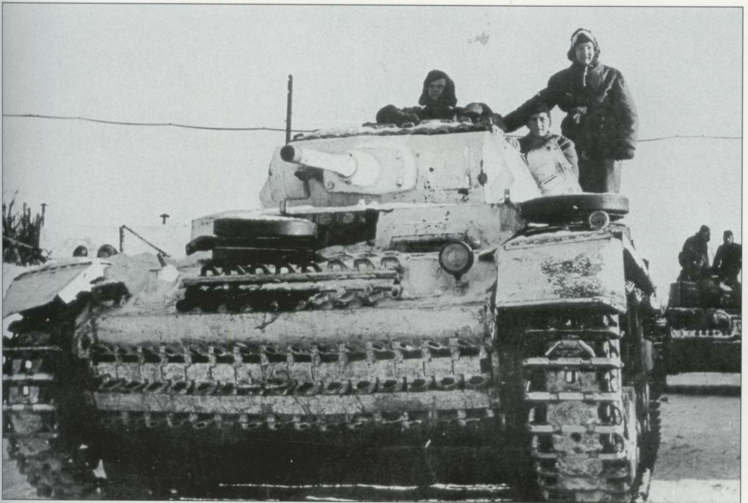
In this photo we see a Pz.Kpfw. III camouflaged with a solid coat of white paint, but behind this tank is a Pz.Kpfw. 38(t) without any winter camouflage. Note that even the tracks fixed to the hull of the Pz.Kpfw. III are painted white.
