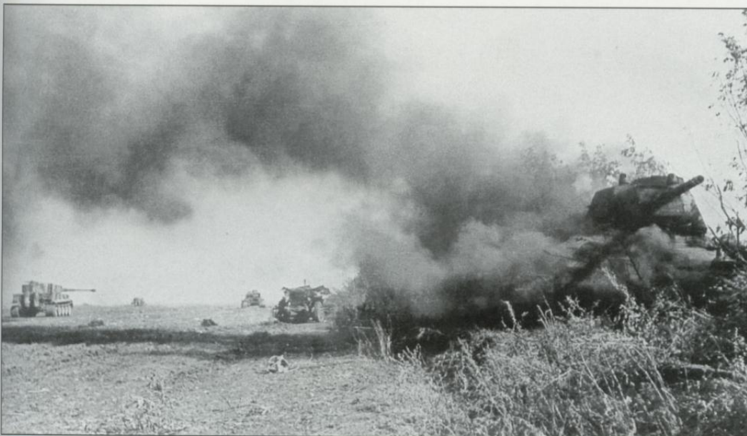
This excellent shot presents a typical picture of an armored attack during Operation "Zitadelle". In the first line are Pz.Kpfw. IIIs armed with long-barreled 5cm guns and equipped with armor skirts (Schürzen) around their turrets. The next line consists of Pz.Kpfw. IV tanks — one of which is visible in the background.
