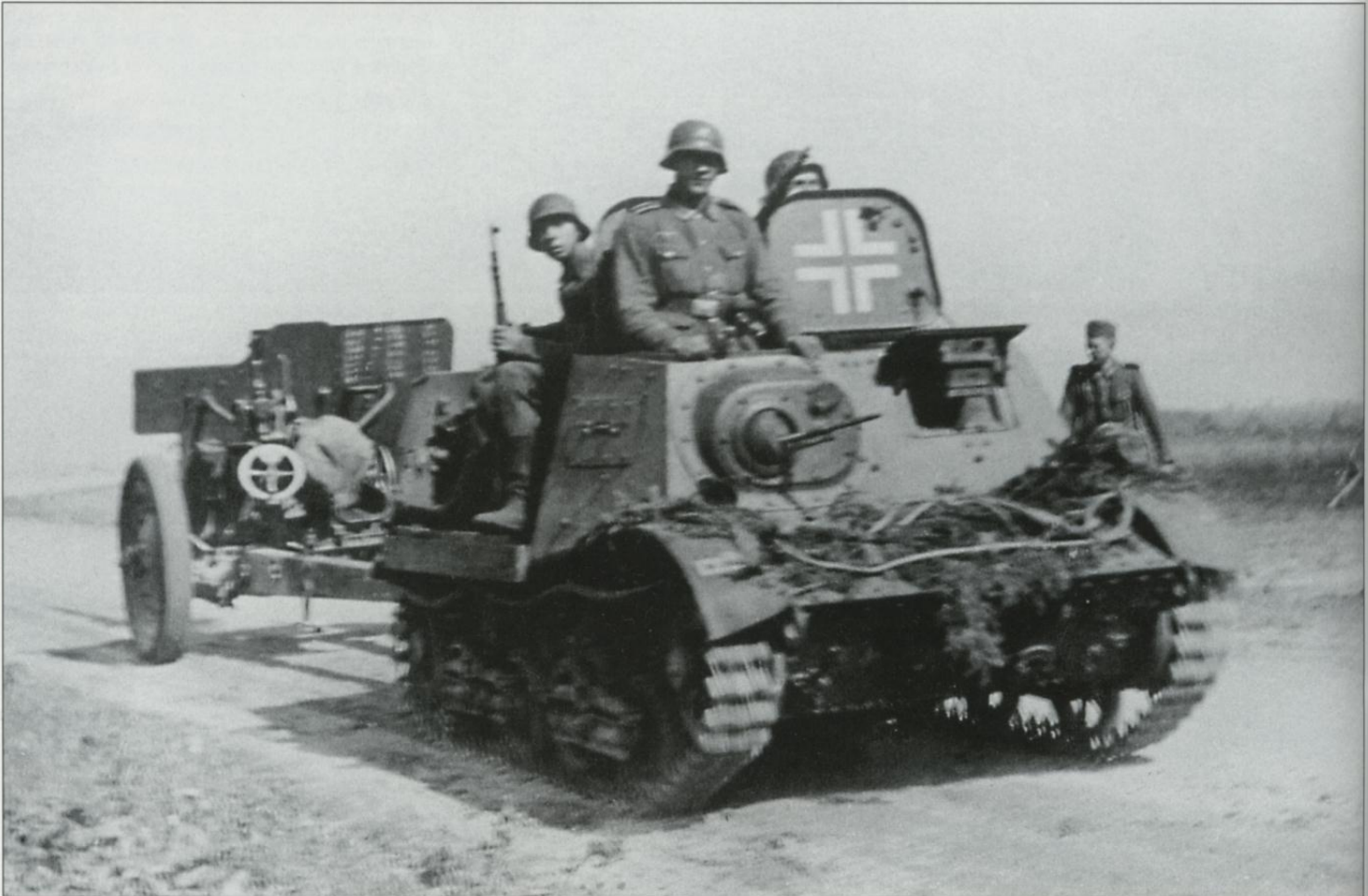
Everything could be useful in the fight against the Red Army, even their own weapons. Here is an example: an armored Komsomolets artillery tractor with a 76.2mm F-22 gun. The victory marks painted on the armored shield of the gun proves that this anti-tank crew was highly effective.
