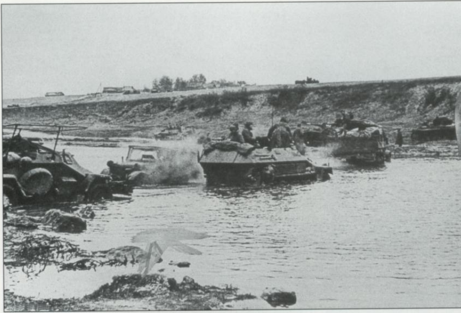
One of the most difficult activities undertaken by the Panzerwaffe units was crossing a river without the help of any bridge and when the river bottom created problems. Suffering most in these situations were soft-skinned vehicles, which were unprepared for such duty. Many of them stalled in the river due to water penetrating the engine compartment.
