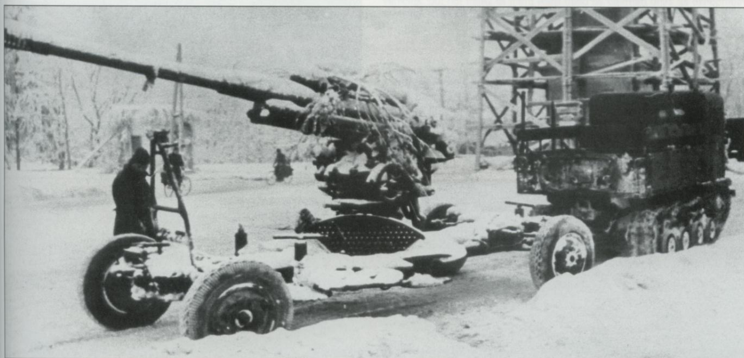
The Soviet equivalent of the German 8.8cm anti-aircraft gun was the 85mm Model 39 gun. Though it was not as deadly a weapon as the German gun, it was willingly used by the German troops. They appreciated the easiness of its operation and found it more powerful than their own 5cm and 7.5cm guns. Here we see a captured full-tracked STZ-5 tractor towing an 85mm gun.
