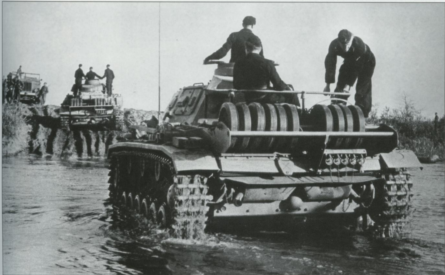
This command version of the Pz.Kpfw. III, the Pz.Bef.Wg. III, was photographed while crossing a stream. Many details of the rear of this type of tank are clearly visible in this photo, including the smoke bomb rack. The most intriguing is the unusual installation of the rack for the spare road wheels on both vehicles. The tractor seen in the background was prepared to help any tank that had problems while traversing the mud.
