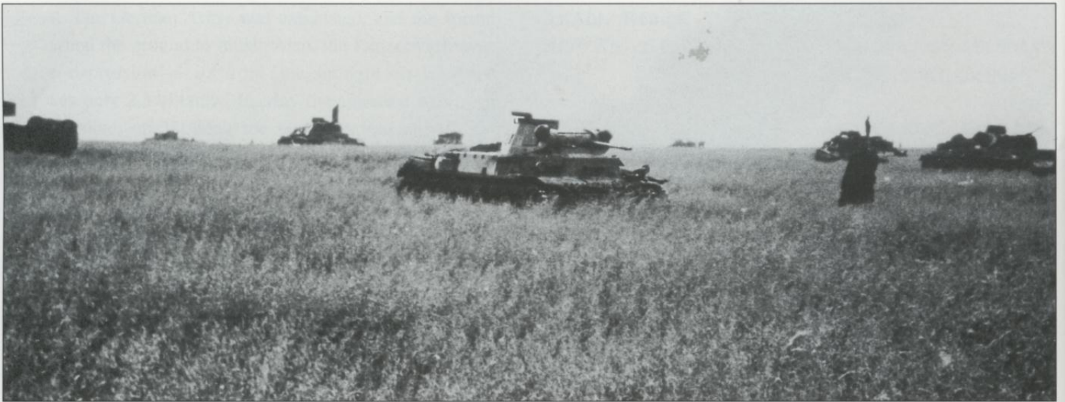
Columns of Pz.Kpfw. IIs and Pz.Kpfw. IIIs wait in a field for the order to attack. In the center of the photo is a Pz.Kpfw. II Ausf. C with an additional box installed on the right side of the tank. There were about 700 of these tanks in front-line units during the opening phase of the war against the Soviets. They were fast, but were not strong enough to be the standard battle tank for the Panzerabteilungen. All of the Soviet standard tanks were better armed than the Pz.Kpfw. II, though this German tank was better armored than the old Soviet vehicles.
