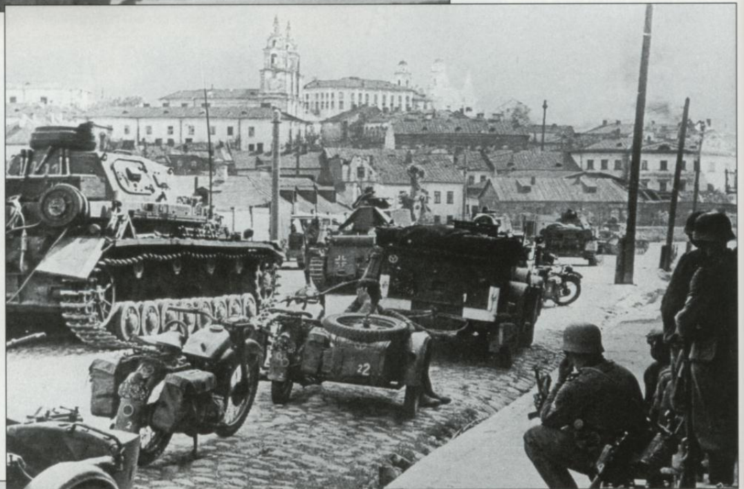
General Harpe's 12.Panzerdivision enters Minsk in the last days of June 1941. Note the Pz.Kpfw. IV Ausf. E at the left, which is equipped with a very rare feature on tanks of this type—the smoke dischargers typical of the Pz.Kpfw. II. The tank is also devoid of a turret basket. In its place are hanging several stick grenades. Also interesting are the markings painted on the rear of the motorcycles. Each of them carries divisional emblems (the one with the sidecar even has two) in yellow and tactical markings in white.
