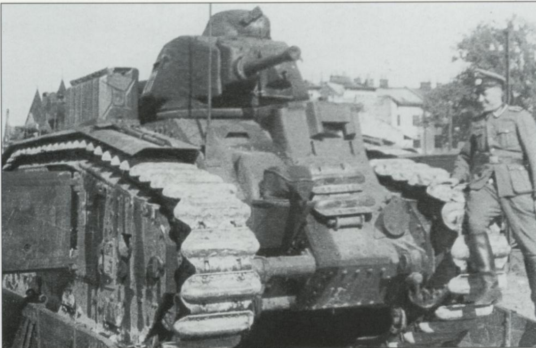
A photograph of a Flammpanzer B-2(f) built on the chassis of a captured French Char B-1 bis medium tank in 1941 and used by s.Pz.Kp.223 during the summer fighting in 1942 in the Crimea. There were twelve of them used in that combat. Note that the tank still lacks tactical markings.
