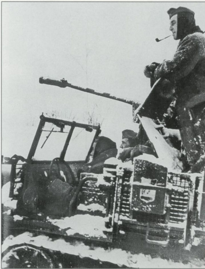
Wide, endless fields of wintertime Russia as viewed from the turret of a Sd.Kfz. 222 light armored car. Note the details of the gun (2cm KwK38 and MG34) installations. The net in the turret top cover is partly eliminated for better visibility.
