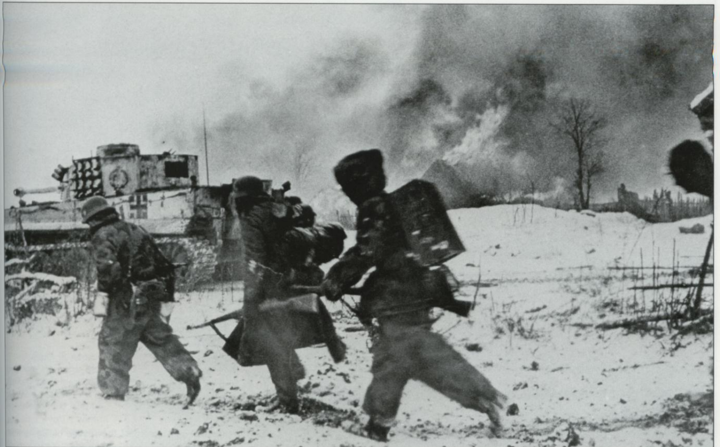
Along with some supporting infantrymen, a Tiger tank moves against an enemy position in a Russian village. Note the style of painting winter camouflage over the tank's original dark gray background — all vehicle markings are untouched by the white paint. This was quite a typical style of camouflage in the Tiger units during their first winter. The Tigers created their first serious problems for the Soviets in the northern sector of the Eastern Front, where s.Pz.Abt.502 was sent.
