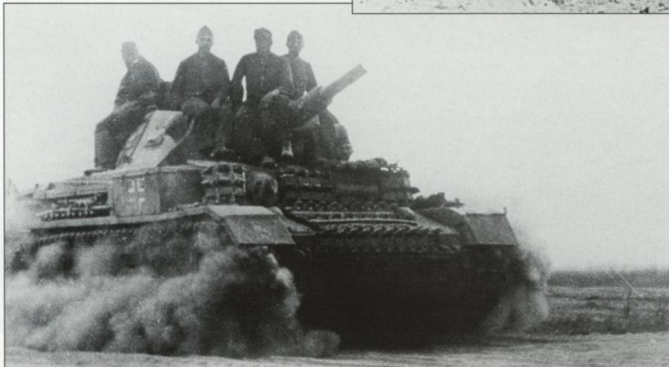
Quite a strange vehicle - probably a Pz.Kpfw. IV Ausf. F2, but without the front half of the barrel and missing a machine gun in the hull position. This tank belonged to 24.Panzerdivision and was photographed somewhere in the Don River bend area in August 1942.
